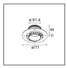
**13642130** Concrete Ring 50 Standard Installation Housing
