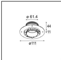
■ **13642130** Concrete Ring 50 Standard Installation Housing
