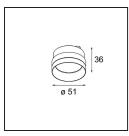
10219930 Reflector 51 Spot Aluminium Anodised
