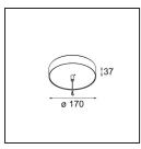
**13523632** Power Feed and Suspension Canopy Surface Round Extruded Trailing Edge DI 350mA (Incl. Suspension Cable 2000) Black Structure
