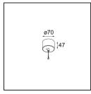
13523132 Power Feed and Suspension Canopy Surface Round 2P Extruded DE (Incl. Suspension Cable 2000) Black Structure
