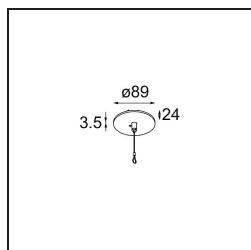
**13523032** Power Feed and Suspension Canopy Semi-Recessed Round 2P Extruded DE (Incl. Suspension Cable 2000) Black Structure
