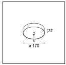
13523232 Power Feed and Suspension Canopy Surface Round Extruded Trailing Edge DI 500mA (Incl. Suspension Cable 2000) Black
