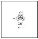
13515630 Concrete Ring 62 Standard Installation Housing
