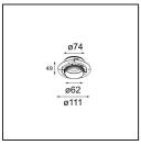
13515630 Concrete Ring 62 Standard Installation Housing
