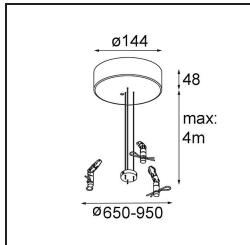
**11066209** Power Feed and Suspension Kit Round 9P Flat Moon (3) Triangle (Incl. Power Feed Cable & Suspension Cable 4000) White Structure
