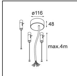
**11062409** Power Feed and Suspension Kit Round 9P Flat Moon (3) Straight (Incl. Power Feed Cable & Suspension Cable 4000) White Structure
