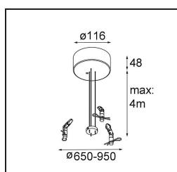
**11066109** Power Feed and Suspension Kit Round 5P Flat Moon (3) Triangle (Incl. Power Feed Cable & Suspension Cable 4000) White Structure
