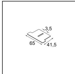
**13271009** Beam Aperture Plate Sulfer Spot White Structure
