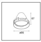
10210009 Reflector 100 Flood Aluminium Anodised
