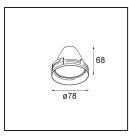
10210006 Reflector 85 Flood Aluminium Anodised
