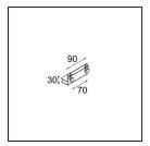
12534009 Mini-Multiple Trimless Mounting Bracket White Structure
