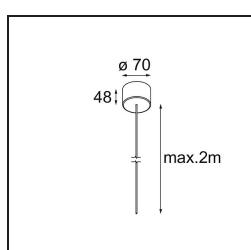
**13720209** Power Feed Canopy Surface DE (Incl. Power Feed Cable 2000) White Structure
