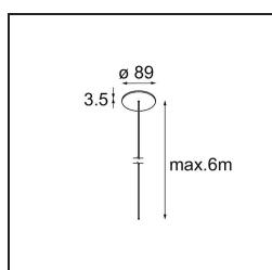
**13720109** Power Feed Canopy Recessed DE (Incl. Power Feed Cable 6000) White Structure
