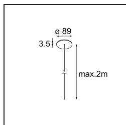
**13720009** Power Feed Canopy Recessed DE (Incl. Power Feed Cable 2000) White Structure
