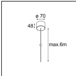
**13720309** Power Feed Canopy Surface DE (Incl. Power Feed Cable 6000) White Structure
