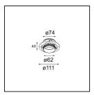
13515630 Concrete Ring 62 Standard Installation Housing
