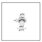
13515630 Concrete Ring 62 Standard Installation Housing
