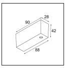
11062732 Power Feed Canopy Surface Square 4P Black Structure11062709 Power Feed Canopy Surface Square 4P White Structure
